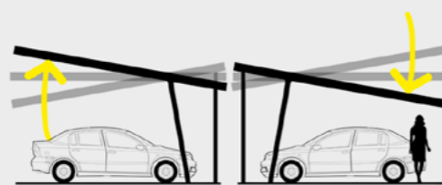
Adaptive roof angle
